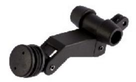
This easy to operate window hold-open is designed to fit comfortably using a two finger operation for top and side hinged venting windows for on and off-highway vehicles. It features an over center design that orientates the window at fully closed and fully open positions and an optional quick release pin in bright red nylon or steel.
